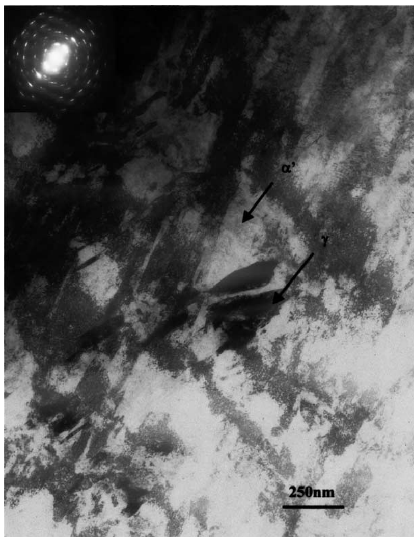
Figure 2 TEM micrograph and selected area diffraction pattern of austenitic stainless steel rolled to 55% reduction in thickness.
